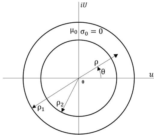
Pic. 1. A case of ring circular air clearance.
