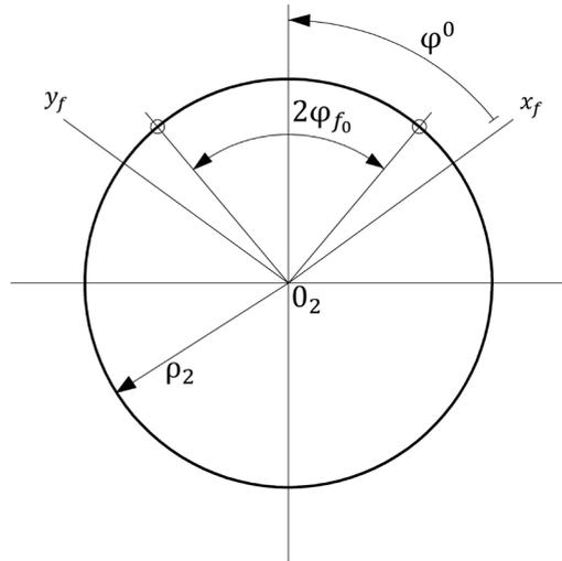
Pic. 4. To the calculation of flux linkage of rotor winding coil.
