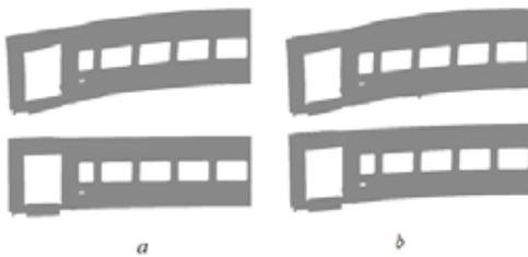
*Pic. 4. Forms of body vibrations on the upper (top) and lower (bottom) FNBV at the equipment frequency of 6 (a) and 9 (b) Hz (author's scheme).*
