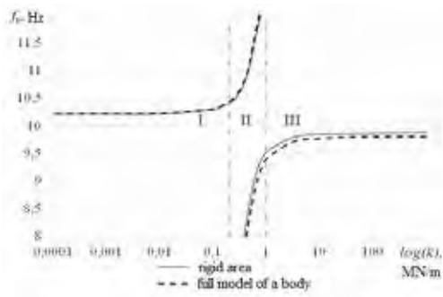
Pic. 2. FNBV with different rigidity of fastening of undercarriage equipment with a total weight of 4400 kg (developed by the author).
