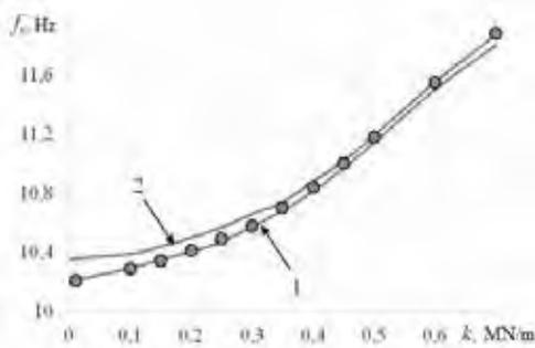
*Pic. 6. Dependence of FNBV on vertical stiffness of the equipment fastenings with absolute flexibility (1), absolute rigidity (2) of fastenings in two perpendicular directions. Markers show the same rigidity of fastenings in three directions (developed by the author).*
