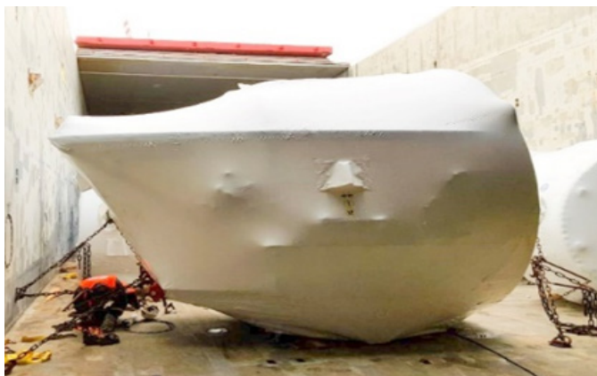
Pic. 3. Securing the nacelle on the vessel (provided by the authors).
