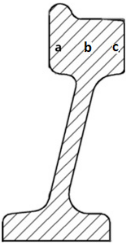
Pic. 1. The main areas of distribution of hardness over the section and on the rolling surface of the rim (compiled by the author).
