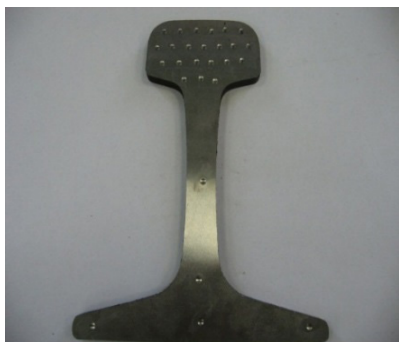
Pic. 2. The template of the rail with indents from the indenters (balls) following Brinell test for determining hardness along the cross-section of the rail [19].
