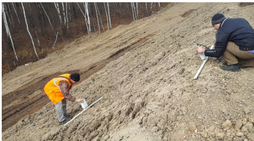
Pic. 8. Conducting GPR multi-offset profiling on a berm slope (provided by the authors).
