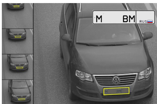
Pic. 6. License plate detection (left) and analysis of car traffic by video image (right). (License plate is partially retouched for publication).
