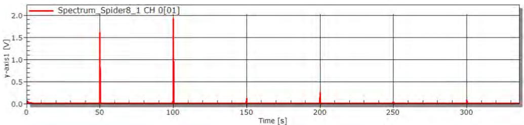
**Pic. 7. DC track circuit (transition from normal to shunt mode, shunt mode and transition to normal mode). Frequency spectrum of the signal at the terminals of track relay when starting from rest [2].**
