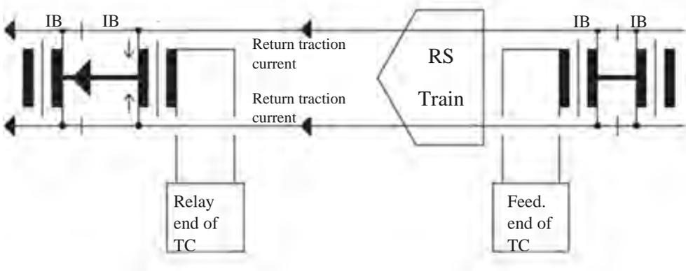
**Pic. 2.** Conditions of electric locomotives testing [1].
