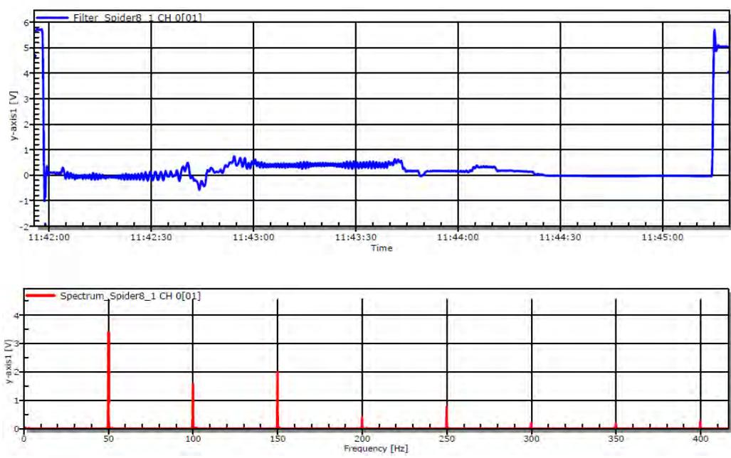
**Pic. 8. DC track circuit (transition from normal to shunt mode, shunt mode, starting from rest and transition to normal mode). Frequency spectrum of the signal at the terminals of track relay [2].**
