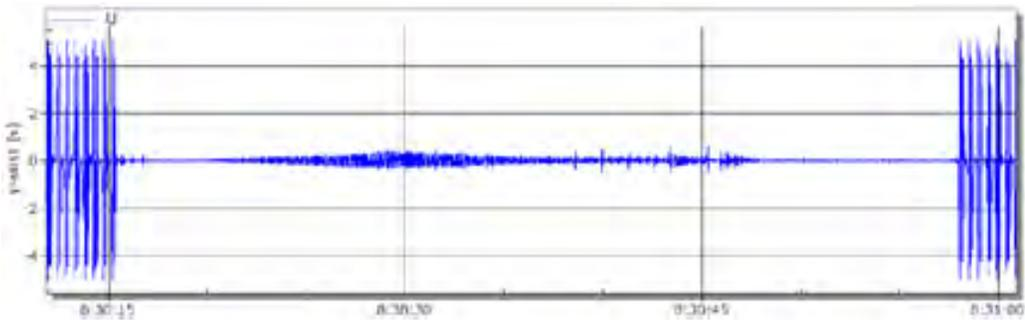
**Pic. 10. 75 Hz pulse track circuit [2].**
