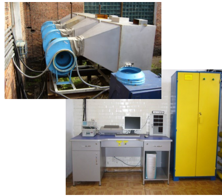
Pic. 2. The diagnostic complex for rheostat tests of locomotives.
