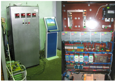
Pic. 1. Automated test stand of rectifier-inverter transformers AC electric locomotives.
