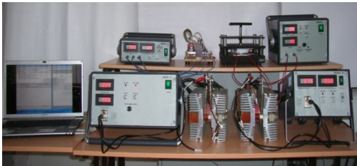
Pic. 3. Complex for automated testing of power semiconductors.
