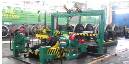
Pic. 4. Technological disassembly position of wheel-motor blocks of locomotives.
