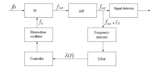
Pic. 3. Scheme of automatic frequency adjustment (automatic fine tuning)  $(f_{int} \pm f_{r})$  through creating control voltage  $\lambda(t)$  and FMO [5], where: M – mixer; AIF – intermediate frequency amplifier;  $f_b$  – frequency of heterodyne oscillator (FMO);  $f_{int}$  – intermediate frequency;  $f_d$  – frequency deviation.
