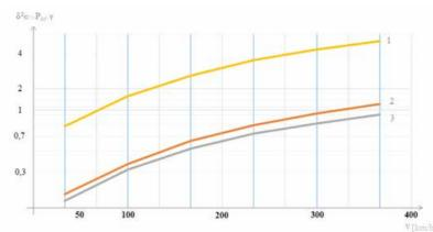
Pic. 4. Dependence of the error  $\delta^2_{,DE}$  (×10<sup>-6</sup>), probability of the error  $P_{er}$  (×10<sup>-7</sup>), efficiency of AIF  $\gamma$  (×10<sup>4</sup>) on train speed V [1 –  $\gamma$ , 2 –  $\delta^2_{,DE}$ , 3 –  $P_{er}$ ].
