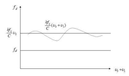
Pic. 2. Graph of change in frequency deviation  $f_a$  (for the case of uneven movement of an object) according to the sinusoidal law with frequency  $M[f_{am}]$  (authors' picture).
