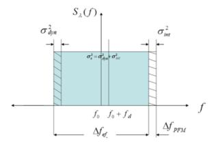
Pic. 1. On the calculation of the reduced dispersion of total error occurred due to the Doppler effect (authors' picture).
