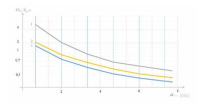
Pic. 5. Dependences of errors  $\delta^2_{\text{\tiny ODE}}(\times 10^{-6})$ ,  $\delta^2_{\text{\tiny AHF}}(\times 10^{-10})$  and probability of the error  $P_{\text{\tiny erAHF}}(\times 10^{-11})$  on the width of the band  $\Delta f_{\text{\tiny alf}}[1 - \delta^2_{\text{\tiny ODE}}, 2 - \delta^2_{\text{\tiny AHF}}]$ .
