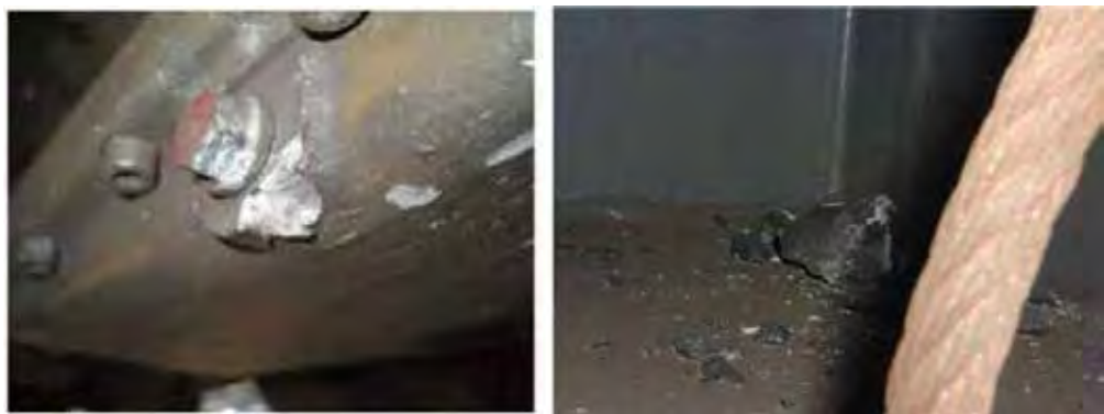
Pic. 1. Damage to the car body from impacts of crushed stone particles [6].
