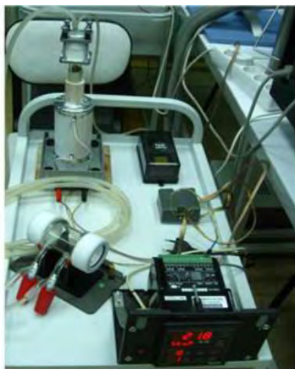
Pic. 4. Temperature-controlled attachment for the study of gaseous products from an insulating material with a calibration cuvette.
