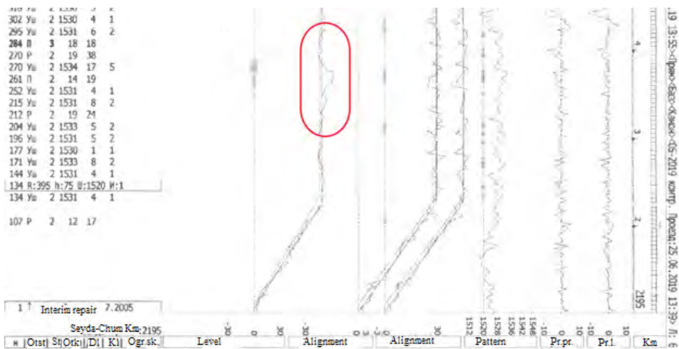
Pic. 7. Graphical chart of the track-measuring (geometry) car (from the archive of Vorkuta Track Division of the Northern Directorate of Infrastructure, graphical chart of the track-measuring car PS067, June 2019).
