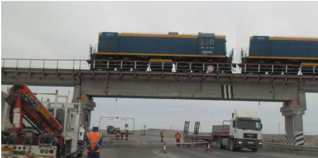
Pic. 5. Authors’ photo of installation of the triple-heading on a span structure 1–2 (load L4).
