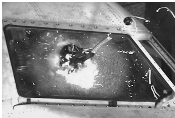
Pic. 4. Air drone breaking through the airliner's windshield during testing [13].
