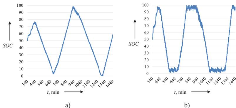
**Pic. 8. Chart of SOC variation for energy storage device at PSK 270: a – with unlimited energy capacity, b – with energy capacity limited to 500 kW·h (authors' calculations).**
