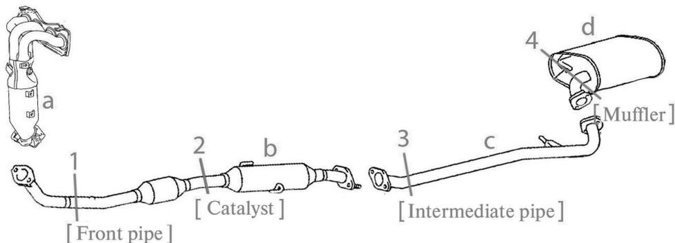
**Pic. 1. Installation points of thermocouples on the surface of the exhaust system:**
