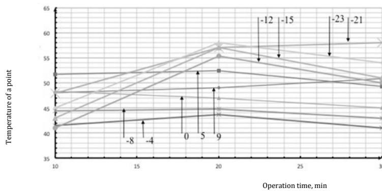
**Pic. 4. Dependence of surface temperature of the elements of the exhaust system on time when the engine is idling; a – front pipe, b – catalyst, c – intermediate pipe, d – muffler.**
