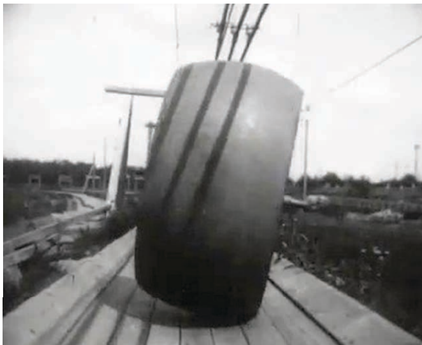
Demonstration of wheel stability. After tilting, it should return to its normal upright position. A shot from the newsreel.
