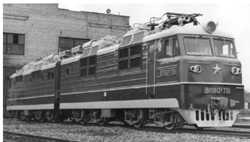
Pilot electric locomotive VL-80A-751.
