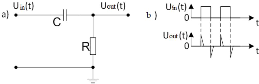
**Pic. 3. Differentiating RC-chain (a), the pulse graph at the inputs and outputs of the chain (b).**
