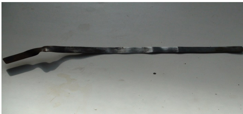
Pic. 5. The test iron plate after immersion in a three-component solution of chloride AIR.
