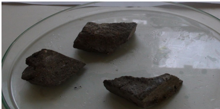
Pic. 2. Concrete samples after five cycles of testing, aged in a 3-component model of an anti-icing reagent.
