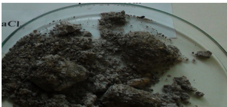
Pic. 4. Concrete samples after 25 cycles of testing, aged in a 3-component model.
