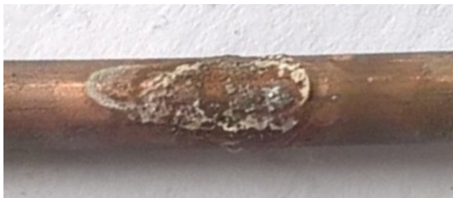
Pic. 8b. Fragment of damage to the sample of copper wire.
