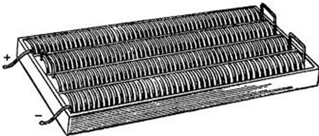
Galvanic battery of Petrov's design. The box was made of mahogany and its length was about three meters.
