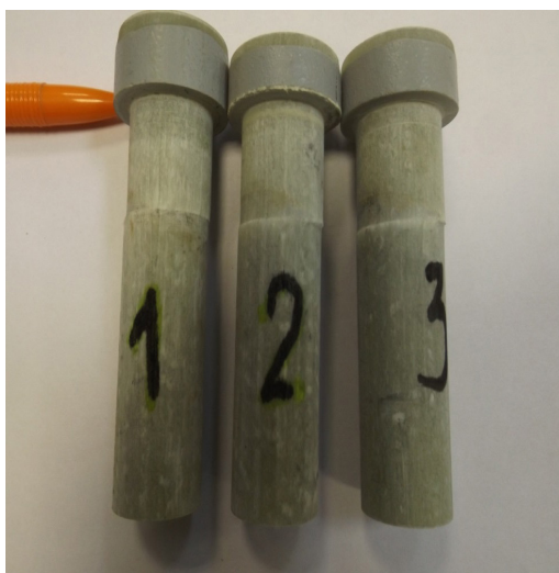
Pic. 4. Samples of composite rollers after testing.
