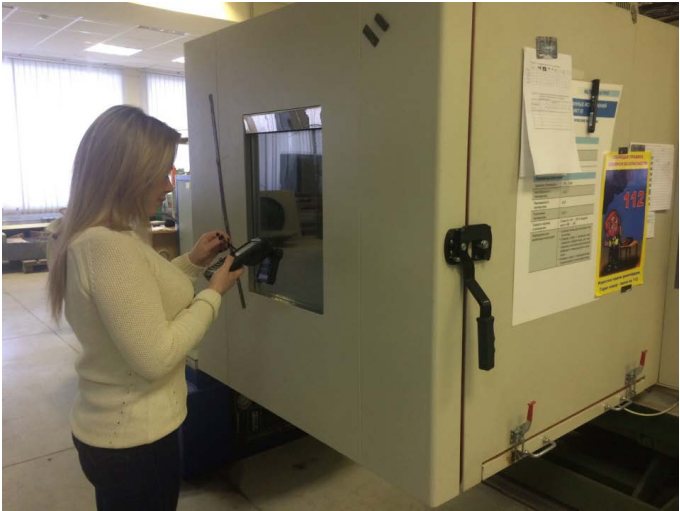
Pic. 2. Experimental tests of RFID-tags in the climate chamber using a portable reader.
