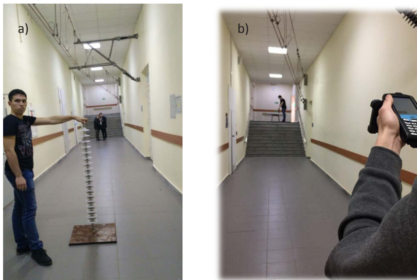
Pic. 8. Conducting experiments to determine range and reading speed regarding samples of RFID-tag on the insulator LK-70–110 with the location of insulators: a) vertical, b) horizontal.
