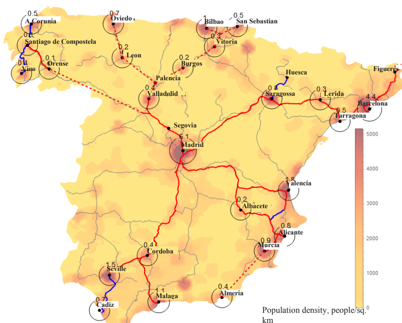
Pic. 3. Network of HSR of Spain. Gray – conventional railways, blue – HSR with a speed of 250 km/h, red – HSR with a speed of more than 250 km/h, dashed lines – under construction (planned) HSR. The population of cities with suburbs (zones surrounded by circles) is given in million people. Compiled by the authors on the basis of the data of the association «Eurogeographics» and [9].
