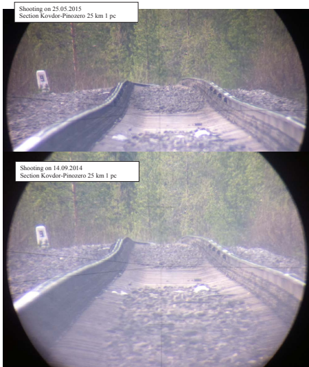
Pic. 6. Relative depressions of the track at the 25 th km of the Kovdor–Pinozero section.
