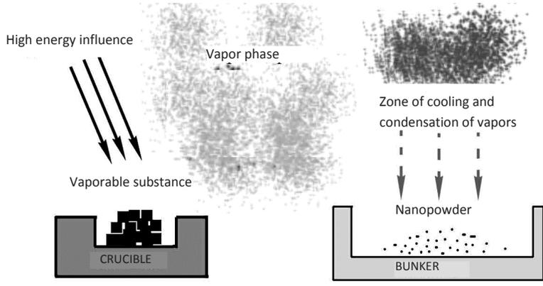
**Pic. 1. Preparation of nanopowder in a chamber with a controlled atmosphere.**
