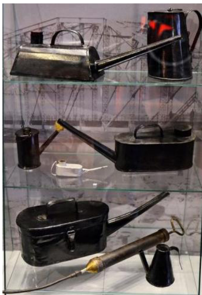
Pic. 8. Typical oiler for lubrication of axle boxes of a steam locomotive and a tender.
