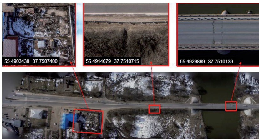
Pic. 3. Orthophotomap of the road section with georeferencing.
