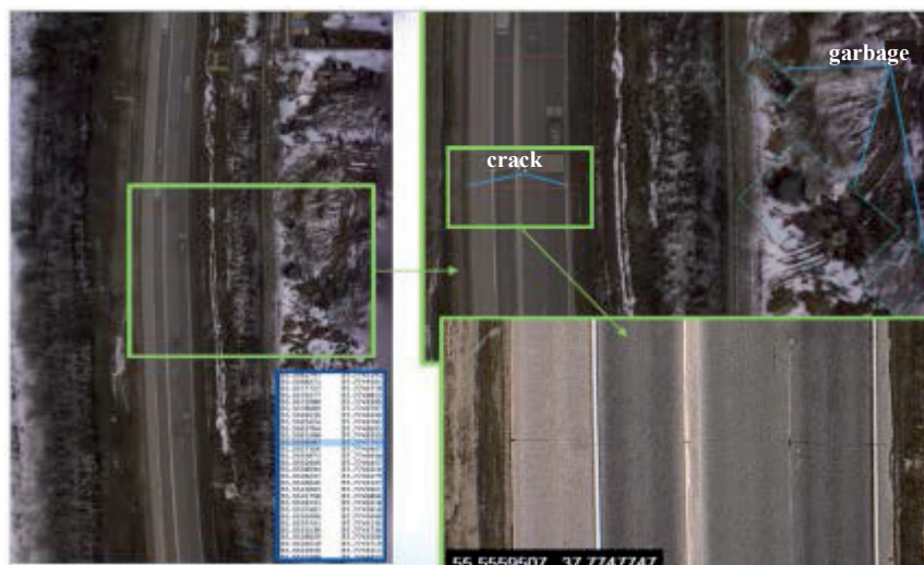
Pic. 4. Transverse defects of the roadway.
