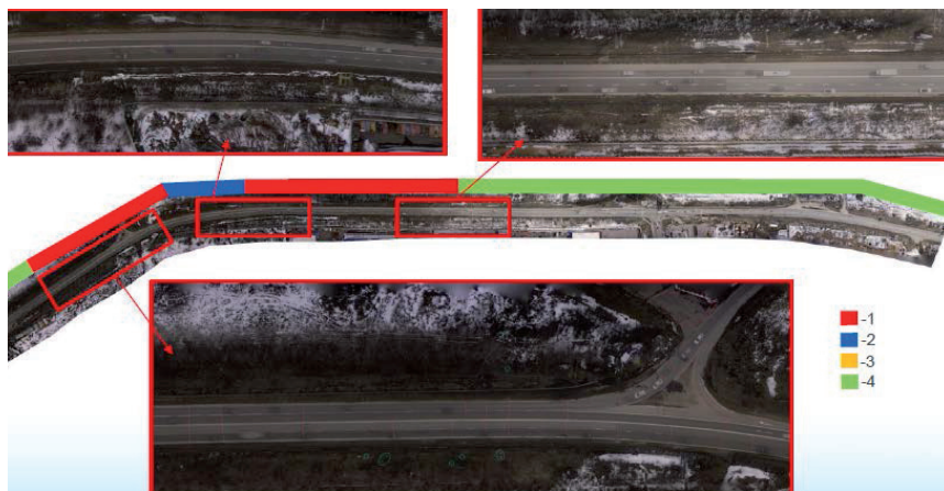
Pic. 5. Distribution of density of defects of a roadway.
