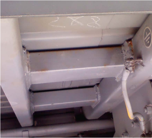
Pic. 4. Car frame reinforced with longitudinal beams.
