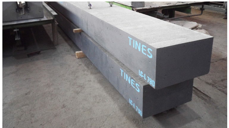
Pic. 8. The plates of the intertrack space of the factory made coating TINES LC-L XL.
