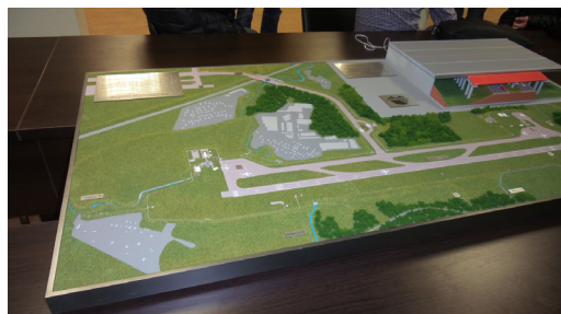
Pic. 2. A design solution for the location of a new runway on the selected section (layout).
