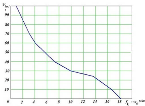
Pic. 2a. Specific accelerating force (in traction mode) 2TE116UM-23AGAL.
