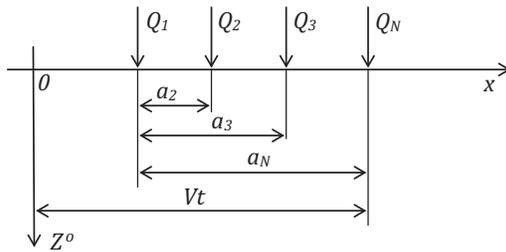
**Pic. 1. Movement scheme of axles' group of a vehicle along the rail.**
