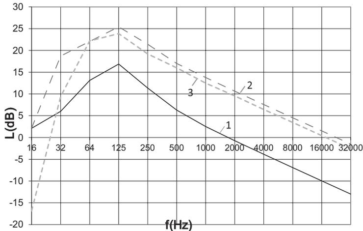
**Pic. 2. Levels of vibration accelerations of a sleeper when axial force is  $N_0=106N$  and vibration damping is  $f_z^0 = 4,5 \cdot 10^4 Pa \cdot s$  (1 – speed 300 km/h; 2 – speed 554 km/h; 3 – speed 700 km/h).**
