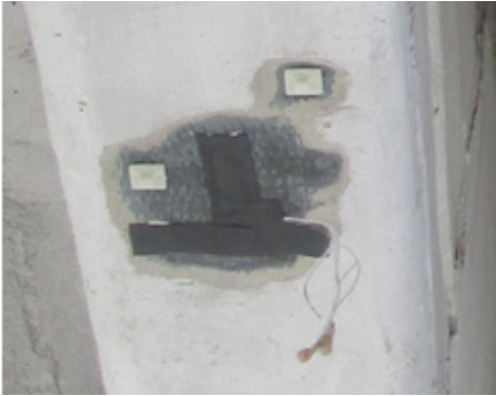
Pic. 2. Strain gauges FLM-60–11 with a protective coating from climatic influences on the lower edges of the edges of the plates.
