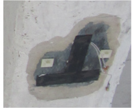
Pic. 2. Strain gauges FLM-60–11 with a protective coating from climatic influences on the lower edges of the edges of the plates.
