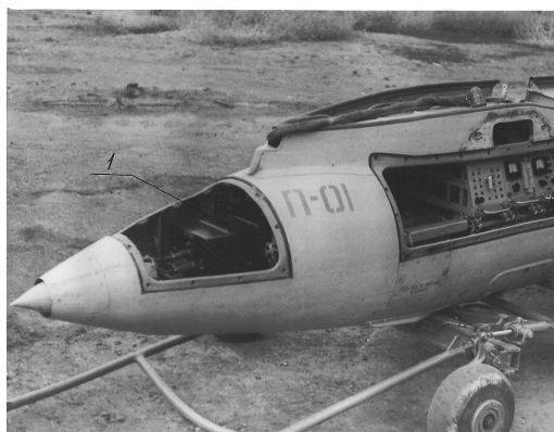
Pic. 1. Allocation of thermal imager «Prostor»: 1 – optical-mechanical assembly; 2 – signal processing and recording assembly.
