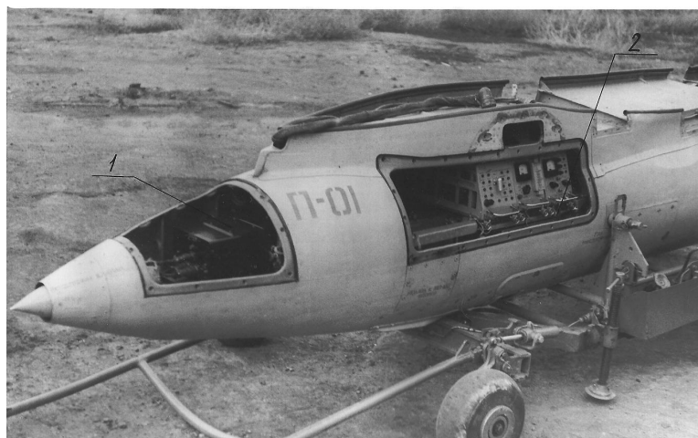
Pic. 1. Allocation of thermal imager «Prostor»: 1 – optical-mechanical assembly; 2 – signal processing and recording assembly.
